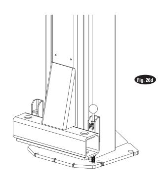
21. Arms & Restraints: Before installing arms, raise carriages to a convenient height. Grease swivel arm pins and holes with Lithium grease. Lift up on spring to allow gear on arm to slide in. Slide arm into yoke, Fig. 26. Install 1-3/4" diameter arm pin(s).
