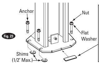
NOTE: Use rectangular shims at inside edge of baseplate. Use constructions adhesive or silicon cement to hold shim in place. INSURE shims are held tightly between base plate and floor after torquing anchors.
