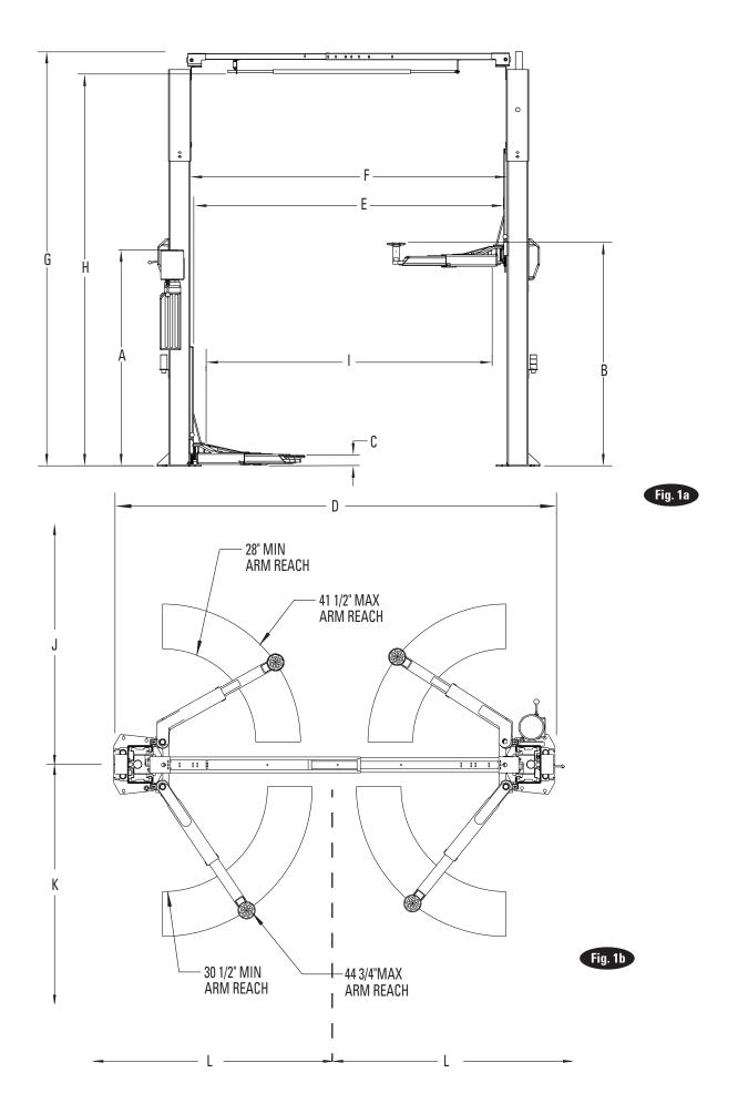
1. Lift Location: Use architects plan when available to locate lift. Fig. 1a & Fig. 1b shows dimensions of a typical bay layout.
