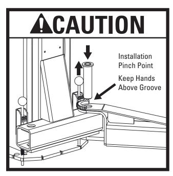
**NOTE**: Once arm is installed in yoke, pull up actuator pin and swing arm fully around, being sure that the Restraint Gear and Gear Block always stay aligned. If they do not stay aligned, remove restraint gear and install in the opposite position.
