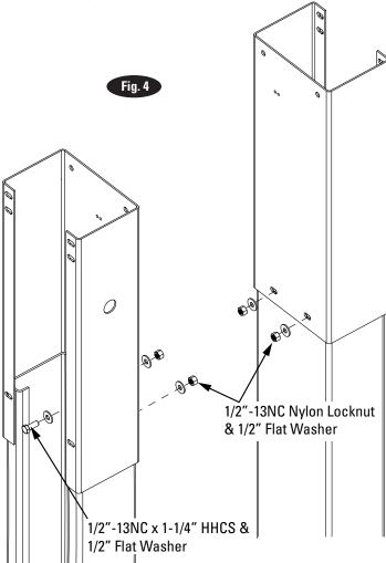
**6. Reinforcement Bar:** Install the reinforcement bar to the column and column extension using (2) 1/2"-13NC x 1-1/4" HHCS, (4) 1/2" Flat Washer, and (2) 1/2"-13NC Nylon Locknut Fig. 5.
