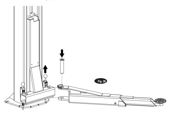
**NOTE**: To check operation of arm restraints, raise carriage 1" min. from full down position. Pull up on pin-ring and adjust arms to desired position. To engage restraint, let pin-ring down allowing gear teeth to mesh together. It may be necessary to rotate arm slightly to engage gear teeth. Tighten nut on actuator pin once restraint function is verified.
